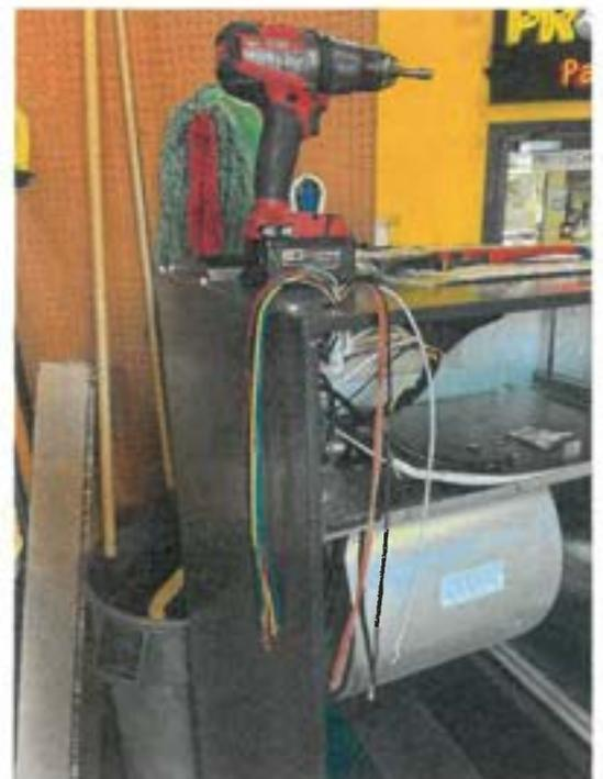
Run all indoor and outdoor wiring from control board through grommet to exterior to meet UL code
